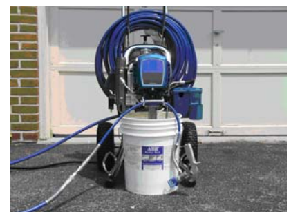
The ABR ® Waterless Cleaning Poultrice can be sprayed with an appropriate airless texture sprayer with a max working pressure of 3300psi, a tip size no smaller than 30/1000 with a delivery rating of 1.1 gpm
